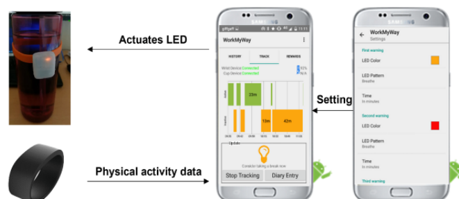
Figure 2. The tracking and prompting component. LED: light-emitting diode.
